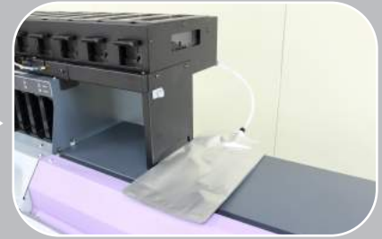
9. Connect a waste ink tube to a spare 2 liter pouch. (This will prevent ink from overflowing when ink leaks inside stand)
