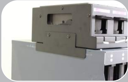
4. Place ink pouch stand on the printer.
