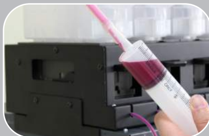
17. Plug the tank again and remove air from the cartridge.
