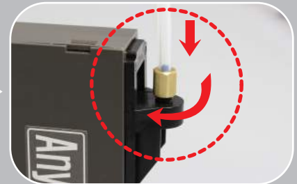
12. Push down an ink tubing to the end, Fasten a nut and plug each cartridge.
