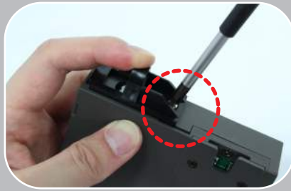
2. Mount a cartridge connector on each cartridge.
