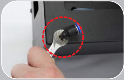
7. Install a fitting on the back side of ink pouch stand.
