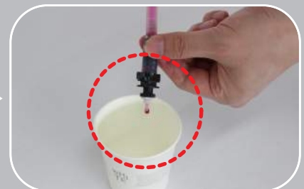
18. Extract ink from air suction kit by inserting an air removing part in the nozzle.
