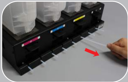
10. Pull out each ink tubing on the bottom.
